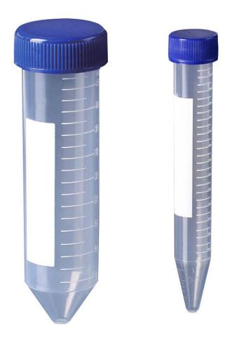
Conical 15mL and 50mL centrifuge tubes are made of premium polypropylene for clarity and centrifugal strength. Tubes and caps may be frozen at temperatures as low as -86°C. The maximum centrifugal force is  $12,000 \times g$  for the 15mL tubes and  $15,000 \times g$  for the 50mL tubes. Caps have a flat top surface for easy marking and labeling.
